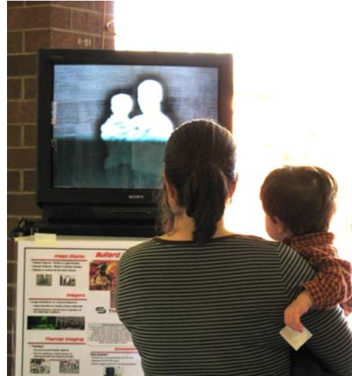
A Thermal Imager is pointed at this mom and child, Their body heat creates an image as seen on the TV screen. Firefighters use this tool to locate people in structure fires.
